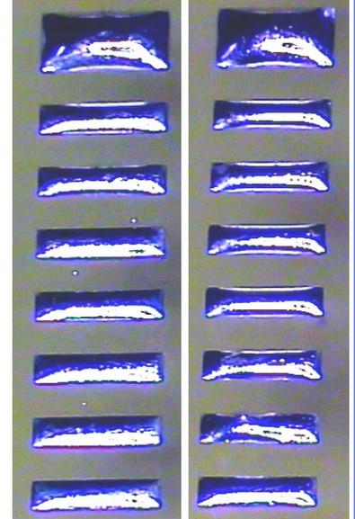
Left: micro solder balls with conventional VOC-free flux
